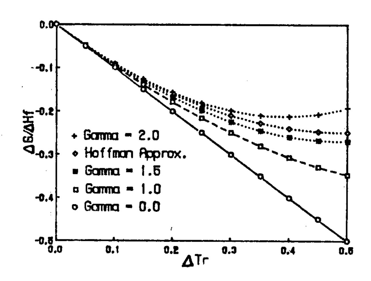
Figure 2. Reduced driving force for crystallization versus reduced undercooling for various values of gamma and for the Hoffman approximation.
