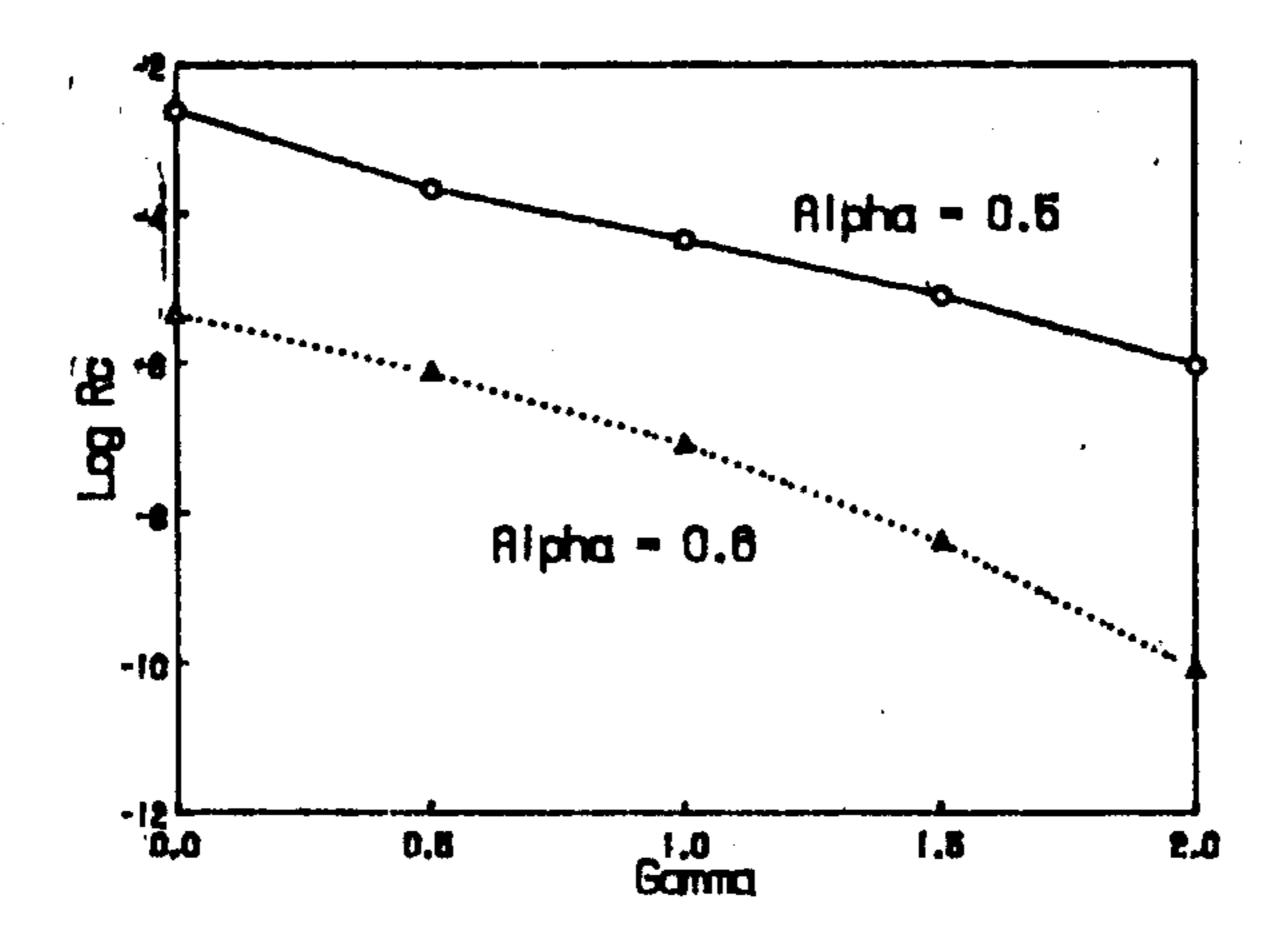
Figure 1. Log (critical cooling rate) versus gamma for SiO2-like material and two different values of the Turnbull ratio (alpha).
