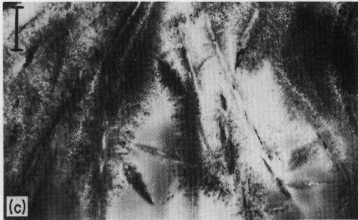
Figure 3 Transmission electron micrographs (100 kV) of thin glass sections. (a) Glass 29.7 H (29.7 mol % BaO) heat treated for 5.5 h at 743°C + 4.2 h at 690°C + 1.0 h at 750°C. The bar denotes 0.1 \mu\text{m} . (b) Glass 28.3 B heated for 30.2 h at 743°C. The bar denotes 1 \mu\text{m} . (c) Glass 29.9 heated for 13.1 h at 752°C. The bar denotes 1 \mu\text{m} .
