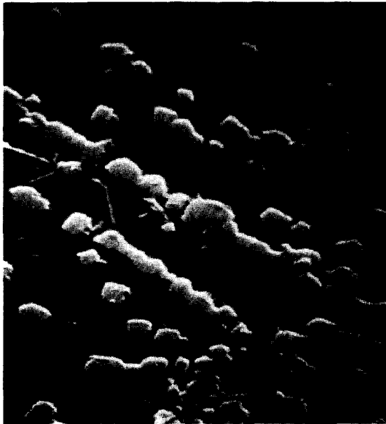
Fig. 1 Square diopside crystals on the surface of diopside glass heated at 820°C. Bar indicates 1 μm.
