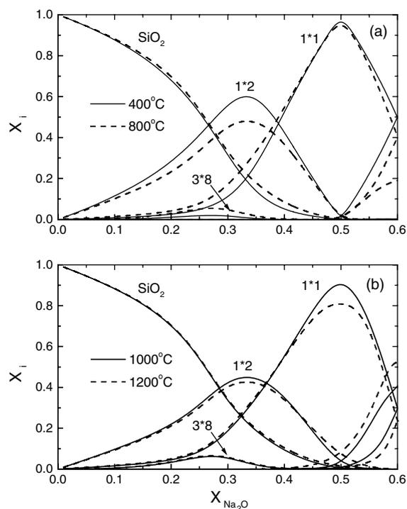
Fig. 1. Chemical structure ( $m\text{Na}_2\text{O} \cdot n\text{SiO}_2$ ) of sodium silicate melts at various temperatures, over the composition region from 0 to 60 mol%  $\text{Na}_2\text{O}$ . (a) Solid line: 400 °C. Dashed line: 800 °C. (b) Solid line: 1000 °C. Dashed line: 1200 °C.
