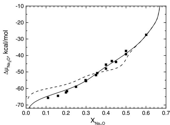
Fig. 4. Chemical potential  $\Delta\mu$  of  $\text{Na}_2\text{O}$  in sodium silicate melts, at  $1200^\circ\text{C}$ , modelled using different sets of species. Squares: experimental data (Ref. [1]). Solid line: calculations considering all salt-like compounds. Dashed line: calculations neglecting  $\text{Na}_2\text{O} \cdot 2\text{SiO}_2$ .
