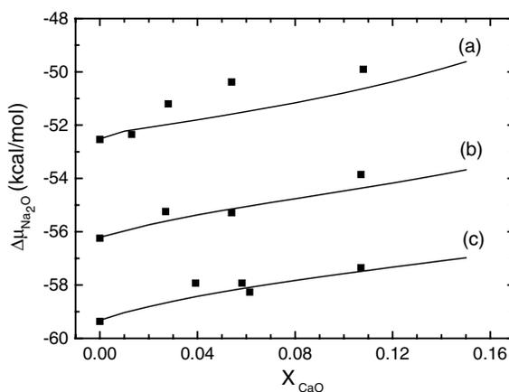
Fig. 5. Chemical potential  $\Delta\mu$  modelled for  $\text{Na}_2\text{O}$  in sodium calcium silicate melts. Solid lines: calculations for different values of the ratio  $\text{Na}_2\text{O}/(\text{Na}_2\text{O} + \text{SiO}_2)$ : (a)  $0.343$ , (b)  $0.294$ , (c)  $0.244$ . Squares: Neudorf's experimental data (Ref. [28]).
