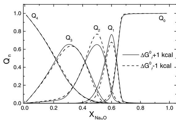
Fig. 2. Evaluation of the variation in calculated fractions of  $Q^n$  species in sodium silicate melts due to a variation on the Gibbs free-energies  $\Delta G_f^0$  of the oxides in  $\pm 1$  kcal around the experimental values (Ref. [18]). Calculations were carried out at 1200 °C.
