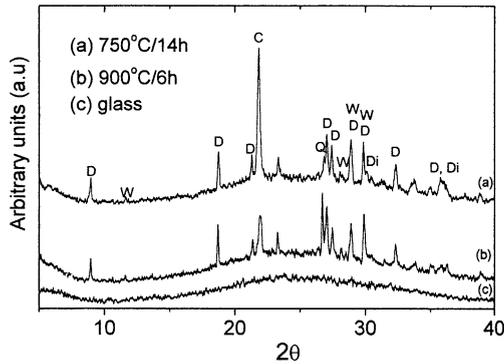
Fig. 7. X-ray patterns of the powdered sample heat-treated at: (a) 750 °C/15 h, (b) 900 °C/6 h and (c) glass spheres as received. D = devitrite, C = cristobalite, Q = quartz, W = wollastonite and Di = diopside.
