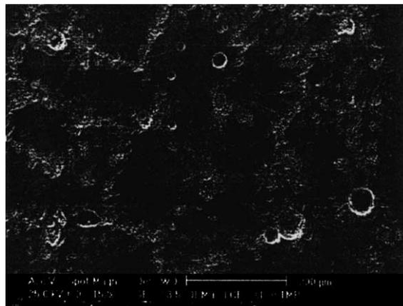
Fig. 13. SEM micrograph of a sample D2 heat-treated at 750 °C/14 h.
