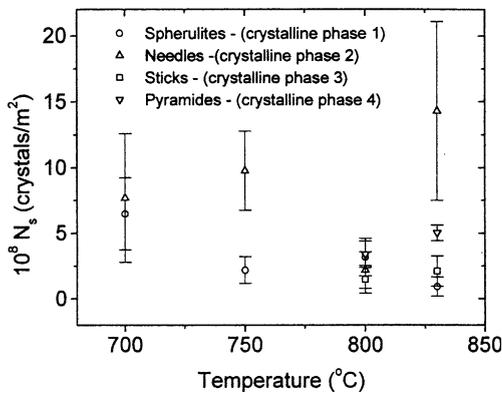
Fig. 6. Average number of crystals per m<sup>2</sup> on soda-lime-silica glass sphere surfaces after treatment at different times and temperatures: 700 °C/5 h, 751 °C/45 min, 800 °C/40 min and 850 °C/40 min.
