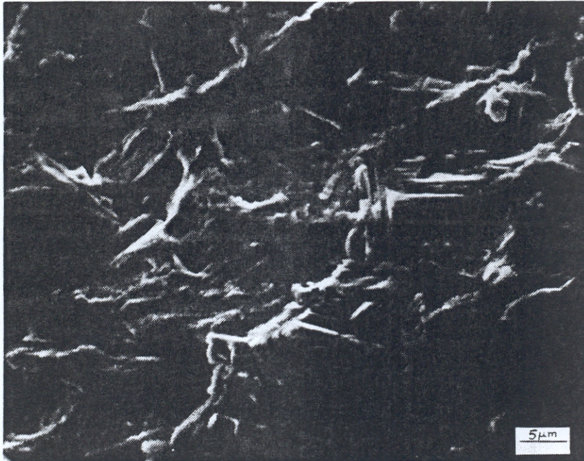
Figure 1a: SEM micrograph of composition 2223 melted in \text{Al}_2\text{O}_3 and cast in a graphite mold.
