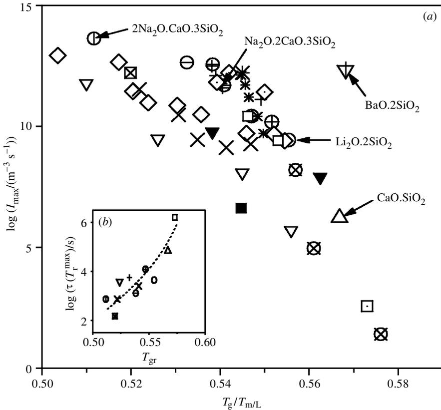
Figure 1. (a) Maximum nucleation rates against  $T_{gr}$  for 51 glasses of stoichiometric compositions and non-stoichiometric compositions. (b) Time-lag of nucleation at  $T_{\max}$ . (After Fokin *et al.* (2002a).)
