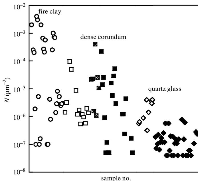
Figure 8. Nucleation density of  $\mu$ -cordierite at cordierite glass surfaces, fractured and annealed under different conditions.  $\circ$  denotes fire-clay furnace, air;  $\square$ , corundum tube furnace, air;  $\boxtimes$ , corundum tube furnace, dust protected;  $\blacksquare$ , corundum tube furnace, dry air;  $\blacklozenge$ , quartz-glass tube furnace, air;  $\diamond$ , quartz-glass tube furnace, vacuum. (Reproduced with permission from Müller (1997).)
