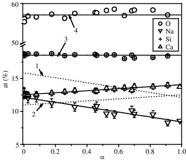
Figure 4. Glass  $1\text{Na}_2\text{O} \cdot 2\text{CaO} \cdot 3\text{SiO}_2$ : compositional variation against volume fraction crystallized at  $650^\circ\text{C}$ . Glass (points) measured by EDS; crystals (dotted lines 1 and 2 denote Na and Ca, respectively) calculated from the parent glass composition and EDS measurements. Solid lines fit the experimental data. Dashed lines 3 (Si) and 4 (O) correspond to the parent glass composition. (After Fokin *et al.* (2002b).)
